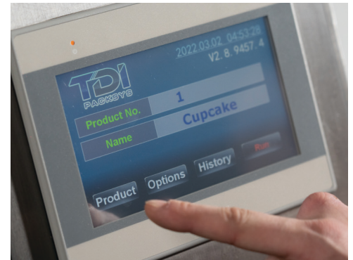
Operator friendly LCD touchscreen HMI – save programs for over 100 products.
