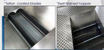
All types of non-stick finishes can be applied. For real sticky doughs, an oil spray system can be fitted where necessary.
