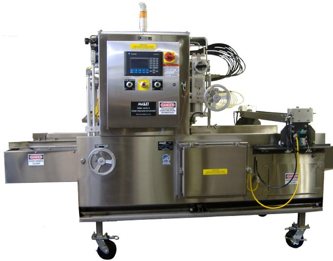
Mallet Model 425 and 435 and 600 Series cake pan greasers are custom designed to produce target area grease application with minimal usage of release agent.
