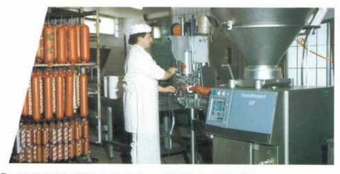
The upper part can be hinged up to provide a gap to observe the level of material in the hopper. A safety switch stops the machine if the upper part is lifted up any further. A hinged step is fitted on the operator side of the VF 200 to give the operator a firm stand and easy access to the two parts of the hopper. The machine does not stop when the step is hinged down but its low height provides a safe footrest.
