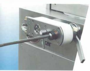
The linking gearbox type 34-4 is easily attached above the worktable. Its rapid coupling secures it firmly to the filler, whilst at the same time the linking gearbox automatically connects with the linking drive. Alignment and tools are not needed.
