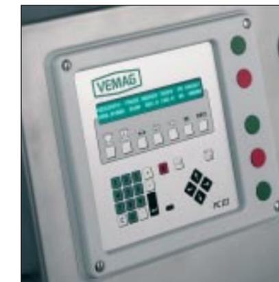
under their names. Set values are entered directly via the decimal keypad of the portioning computer and accepted with a single key. Weight corrections can be entered directly in grammes. All outputs are displayed in clear text in the desired language. The VEMAG Online net program package allows the portioning computer to be connected to one of the plant's master computers – and with a modem extension, to VEMAG Customer Service.
