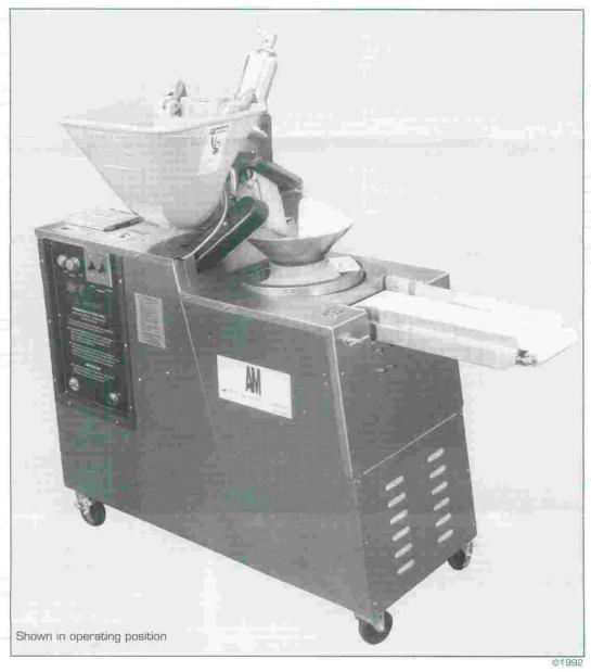
The Atwood Scale O Matic is a single pocket divider/rounder that will accurately divide over a broad range of sizes, then produce a round of unequaled quality, to the greatest variety of baked goods in the industry.
