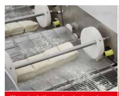
Water depth / immersion depth can be set separately for each water bath
