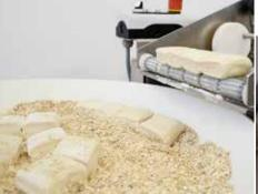
Transfer directly into a rotating bowl with the respective spreading material
