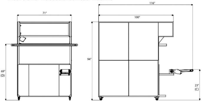
\*Please note that the 640 pocket intermediate proofer's entrance is located in the back side and dough pieces fall down to the moulder from the front side, making the 640 faster than other models.
