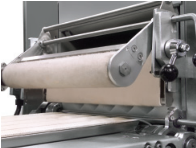
Liftable dough discharge roller for transfer with seam down
