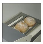
Rear loading belt Provides uniform continuous cutting, thanks to adjustable side guides.
