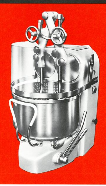
The double arm mixer employs a most gentle mixing action through the use of two stainless steel arms which move with an elliptical motion into the revolving stainless steel bowl. This results in a kneading motion that duplicates "hand mixing" which makes the "Duo-Flex" especially adapted to mixing pie dough and soft sweet doughs.
