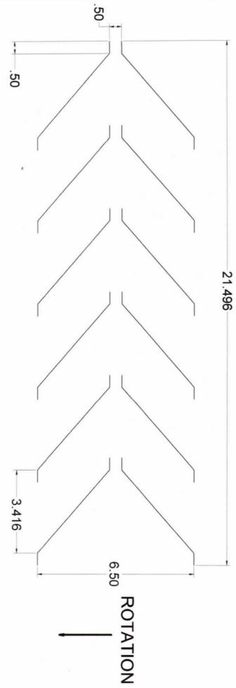
STRIP CUTTER IS 75 TOOTH GEAR DISC. DIA. 152mm CENTER HOLE DIA. TO FIT HUB IS 40 mm BLADE THICKNESS .036
