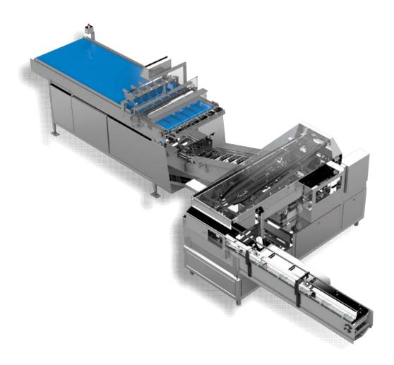
LMC's BB19 Bagel bagger provides unmatched quality and reliability for our customers around the world. With ability to produce 60 bags per minute with superior laning, grouping, orientating, feeding and bagging makes this the best complete line on the market.
