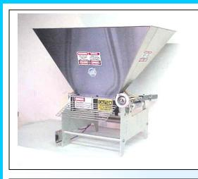
Tabletop stand-alone depositors available in 4, 5 or 6 piston units. Muffin production from 700 to 1,000 dozen per hour with a minimal amount of space used. This fourth generation machine is virtually maintenance free. Tabletop depositors are ideal for feeding rack ovens.
