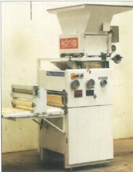
Rex Automat 5-pocket, with dough hopper TRM 160 and spreading finger belt duster.
