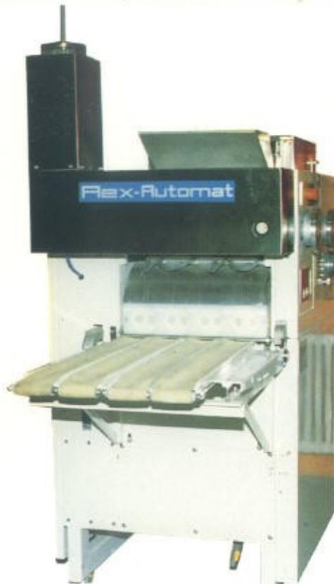
Rex Automat with fitted oiling unit.
