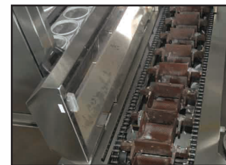
Teflon Coated Loader Buckets
