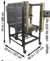
Compressed Air 10 CFM @ 90 PSI Electric 230V, Single Phase, 20A
