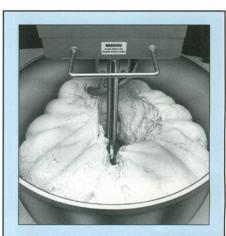
Breaker Bar Mixing and close spiral-to-bowl tolerances yield complete development of large and small batches.
