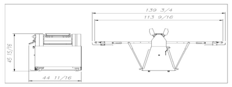
Electrical: 208/220 Volt 3 Phase 60 Hz 12 Amps. Supplied with twist-lock plug. Recommend a 15 Amp slow-blow breaker. Plug: NEMA L15-20P
