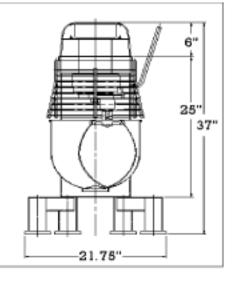
Electrical: 115 Volt 1 Phase 60 Hz 12 Amps 1.5 HP. Supplied with grounding plug.
