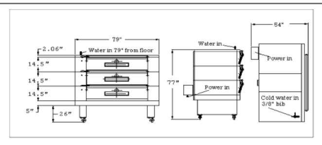
Electrical: 208/220 Volt 3 Phase 60 Hz 84 Amps 30 Kw. Recommend a slow-blow breaker\*
