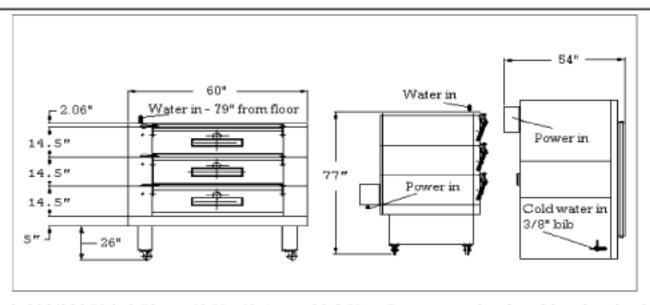
Electrical: 208/220 Volt 3 Phase 60 Hz 62 Amps 22.2 Kw. Recommend a slow-blow breaker\*
