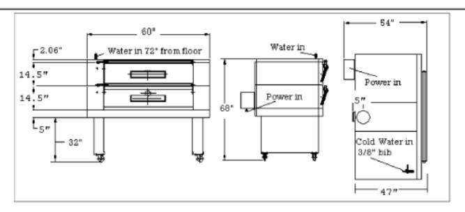
Electrical: 208/220 Volt 3 Phase 60 Hz 45 Amps 14.4 Kw. Recommend a slow-blow breaker\*
