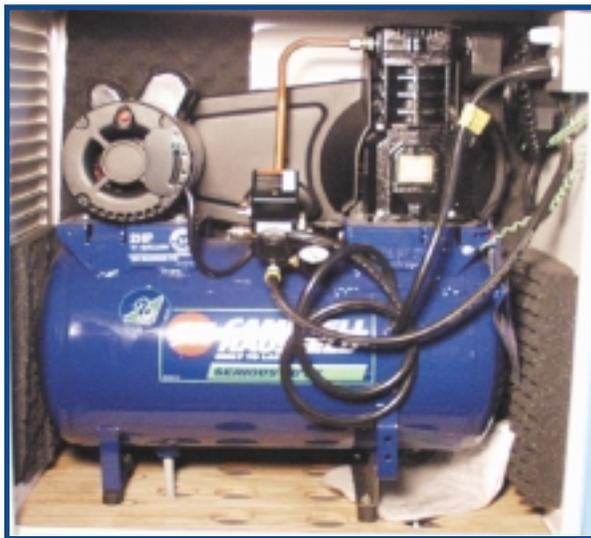
**Features include:** Auto On / Off switch, compression regulating valves, emergency release valve, reset button and a custom fitted drain valve.
