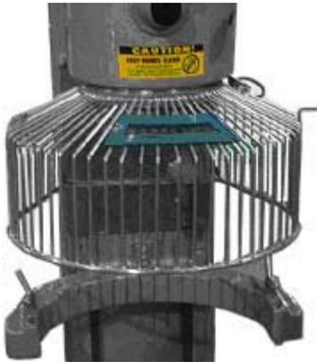
Push guard to the very top of the planetary and tighten. Place bowl into machine and lift to the upper limits to make sure the guard is in the correct position and has some clearance between the bowl and the guard.
