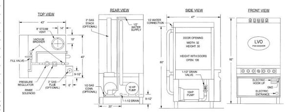
NOTE: Dimensions Marked with \* are 2-1/2" lower on electric heated machines
